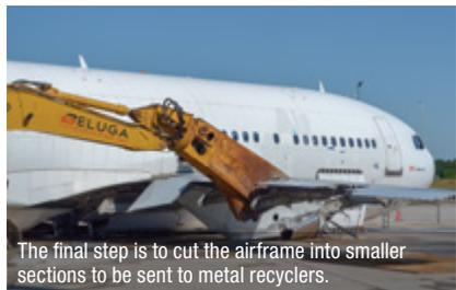
The final step is to cut the airframe into smaller sections to be sent to metal recyclers.
